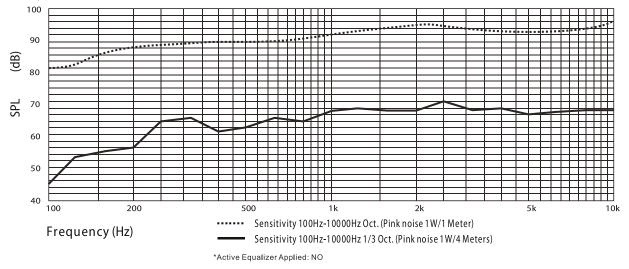
The MCS20T/EN & MCS20T/ENC have been tested for 100 hours at a maximum power of 20W. Both units did not deviate by more than +/- 3dB. The frequency response and impedance curves remained constant throughout the test period. All results are in full compliance with the requirements of EN54-24
